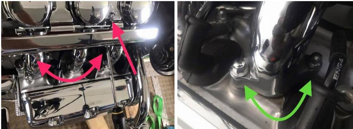
(left) 1st thing I do is to remove the chrome covers off the choke slides. Not worth scratching and it makes it so much easier to remove the intake runner bolts. By removing these it allows you to be able to use a long extension down to the bolts to remove them very easily. Worth the 3 little screws it takes to remove them
