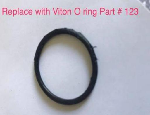
(left) Turn it over and you'll see the o ring that needs to be removed and replaced. Clean the surface real good before putting the new o ring on. Just above the red arrow you see a little nipple sticking out, make sure the passage is clean inside these also. Depending if your bike has been desmogged or not you may have some lines still to connect to them. But even if they are capped it's a good idea to clean them so if you decide to sync the carbs it will be clean.
