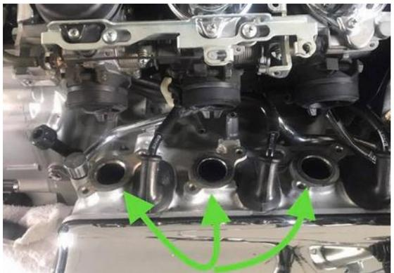
(left) Once all are removed and the holes are plugged I clean the mating surface real good for a tight fit. I smear a little Vaseline around the holes to help the runners slide back in when I replace them
