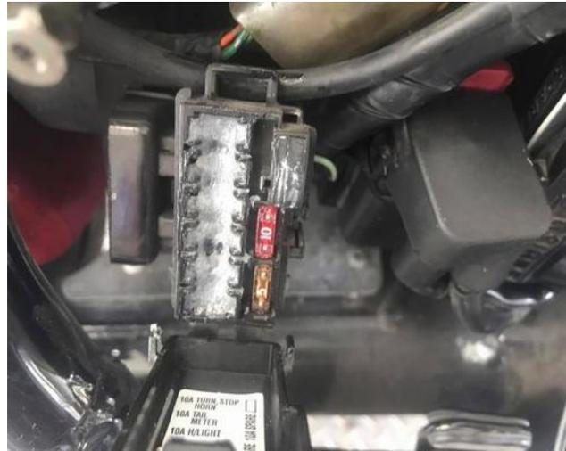
(left) I use my pocket knife to scrape the corrosion of the fuse blades so they make the best connection possible
