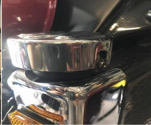
(left) Remove the radiator cap from front right side of bike
