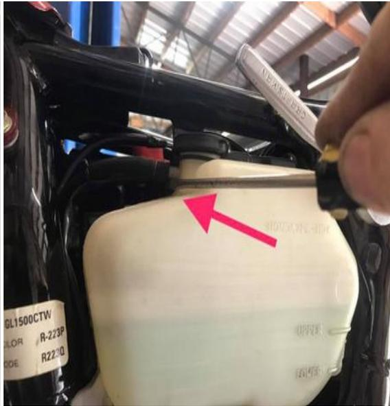
Next push the vent line off the top of the tank. Use caution not to break the nipple off the tank, it is plastic.
