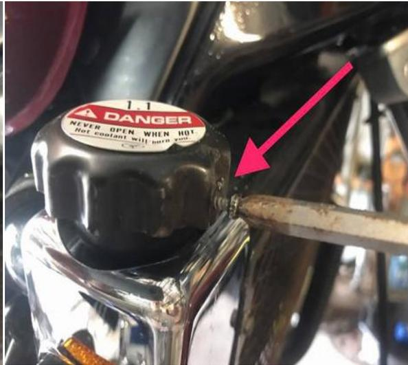
(left) Chrome cap is just held on by double sided tape so should pull off or pry a little up on it thru the opening by the Phillips head screw to get it started.
