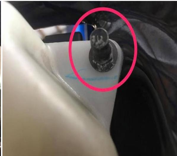
(left) Next we have to remove the reservoir bottle behind the Left side cover under the seat to drain and clean it.
