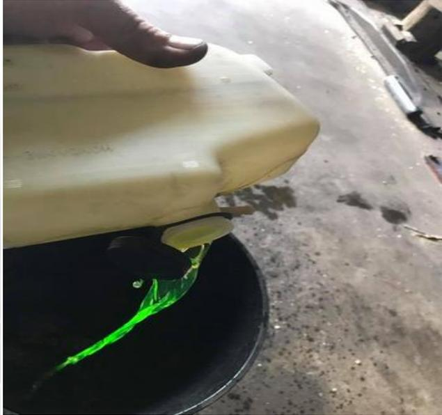
(left) I use a screwdriver and pry it off, it will usually come right off without even messing with the wire clamp. Be careful not to break off the plastic nipple on the tank trying to force it though.
