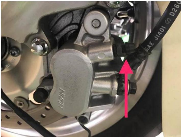
Locate the bleeder nipples on the calipers. I always start with the farthest one which would be the left side then do the right. 2 calipers on the front brakes
