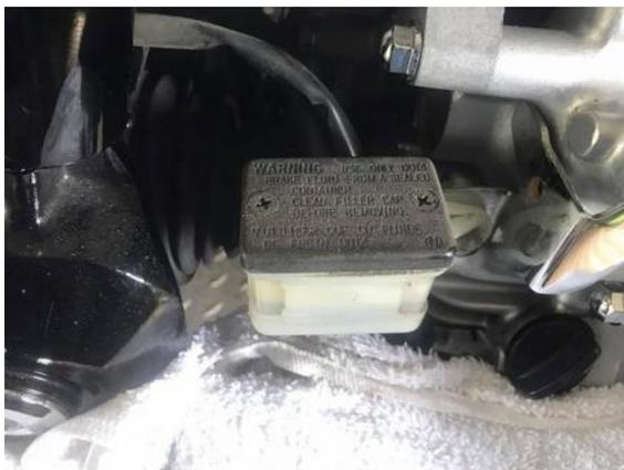
Once the cover is off remove the 2 Phillips screws and cap.
