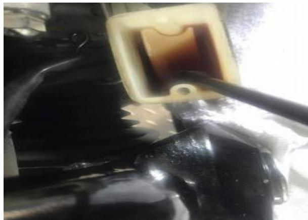
Under the cap is another cap and rubber diaphragm and plastic float. Remove old fluid with a syringe.
