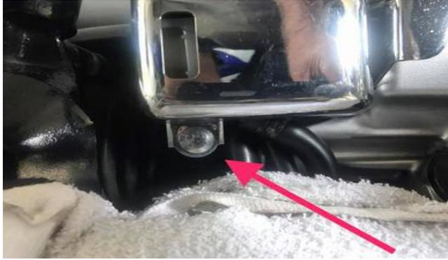
The rear brake master cylinder is down behind the right side foot peg. Remove the 8mm bolt under the chrome cover to expose it.
