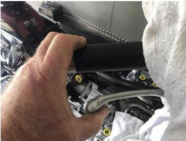
Pump the brake handle up so you have solid brake and hold it.
