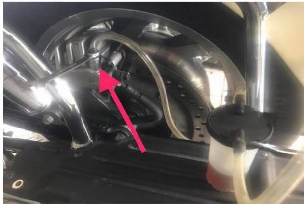
Locate the bleeder nipple on the back left side of the wheel. Add the 10 mm wrench and tubing to the nipple
