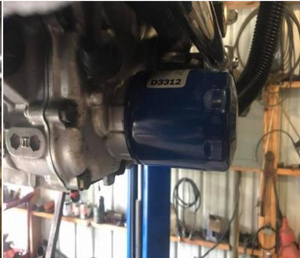
(right) Locate the oil filter on the front of the motor.
