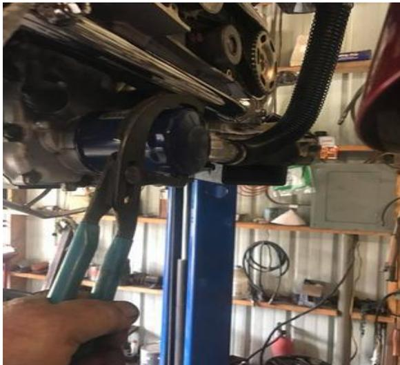
(left) Loosen the filter with an oil filter wrench
