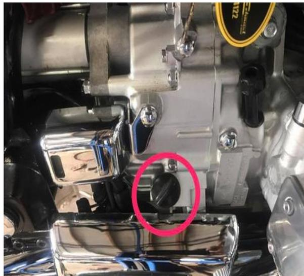
(left) Install the drain plug back in, only takes like a 1/4 grunt torque. Go easy.
