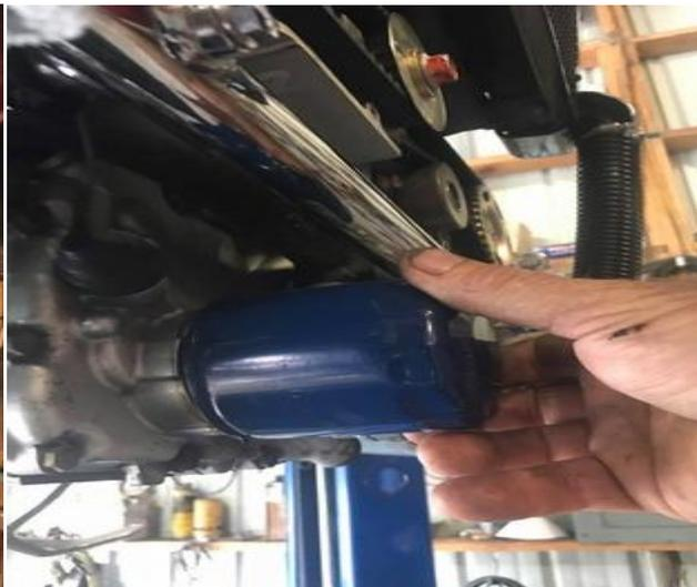
(right) With drain pan to under the filter and take it off.
