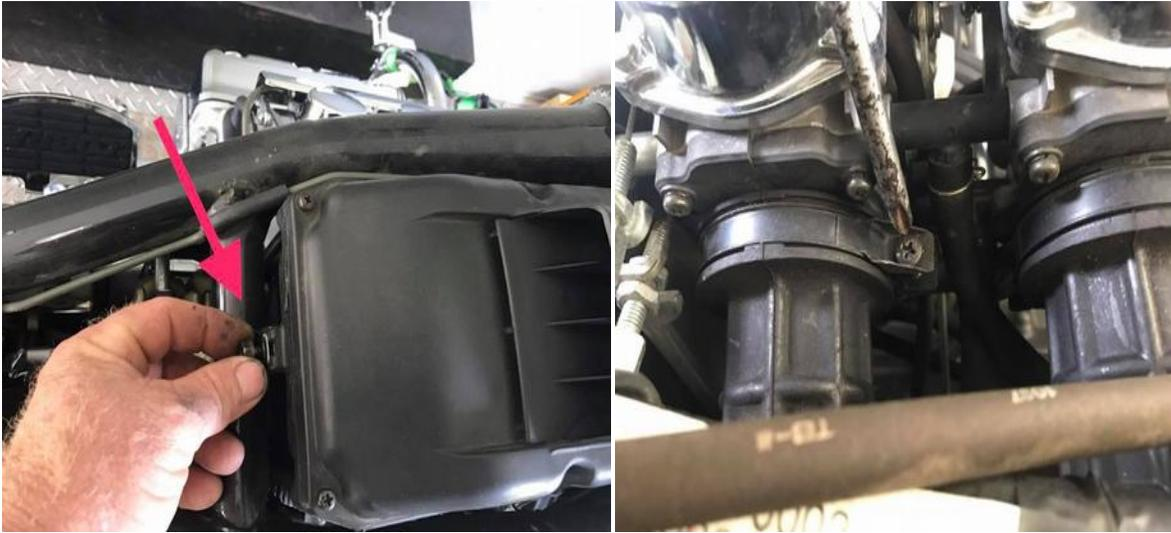
(left) Remove the bolt at the back of the airbox
