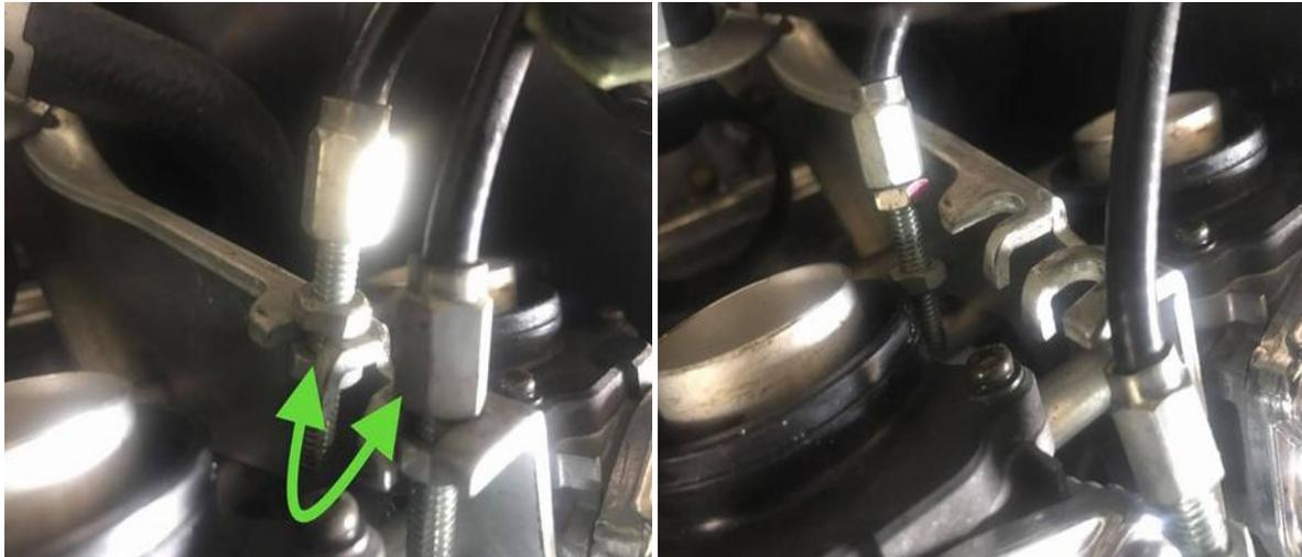
(left) Loosen the adjusters so you can get the cables out of the holders to make slack to release the throttle cables. You can mark the settings with paint or a marker if your unsure on how to adjust them when putting back together.
