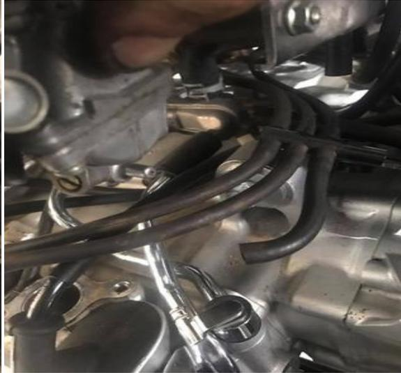
(left) There are 6 carb drain lines that attach to the carb bowls and come to a T. Remove the line at the T
