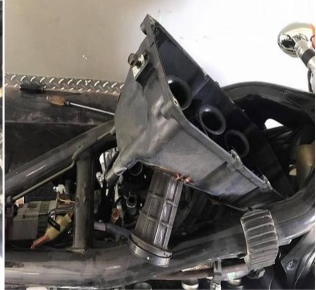
(left) Start lifting the back of the box out while making sure the tubes are coming free from the carbs. Don't worry if the clamps come off you can get them once the box is out of the way.
