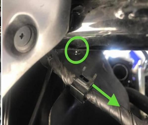
(left) 3 bolts and a tube from the drool tank gets removed to get the right side motor mount off.
