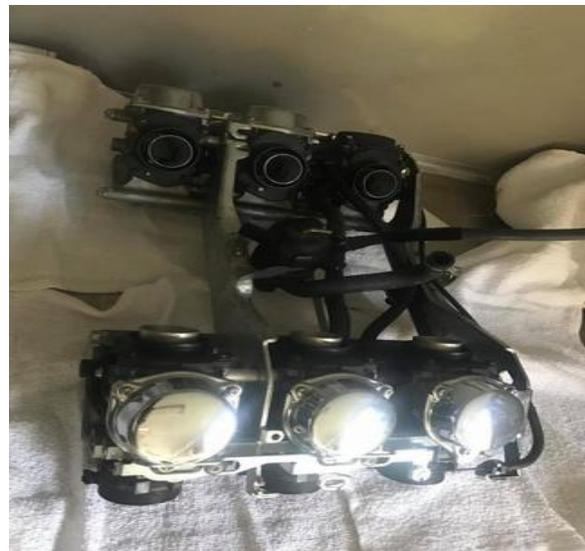
(left) Start working the carb assembly out the left side. Go easy and watch for hoses and wires that may try to get tangled in them.
