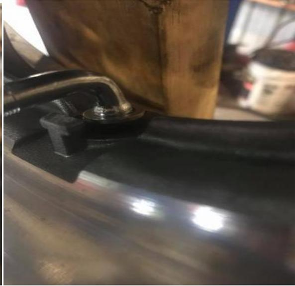
(right) 2nd the metal washer, push it down as much as you can to make room for the nut to fit on.
