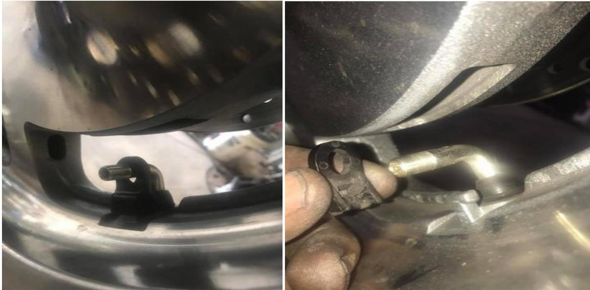
(left) This is a OEM stem, the metal part of the stem stops right where it meets the rim. They put a little plastic crutch under it to keep it from breaking off 😏.
