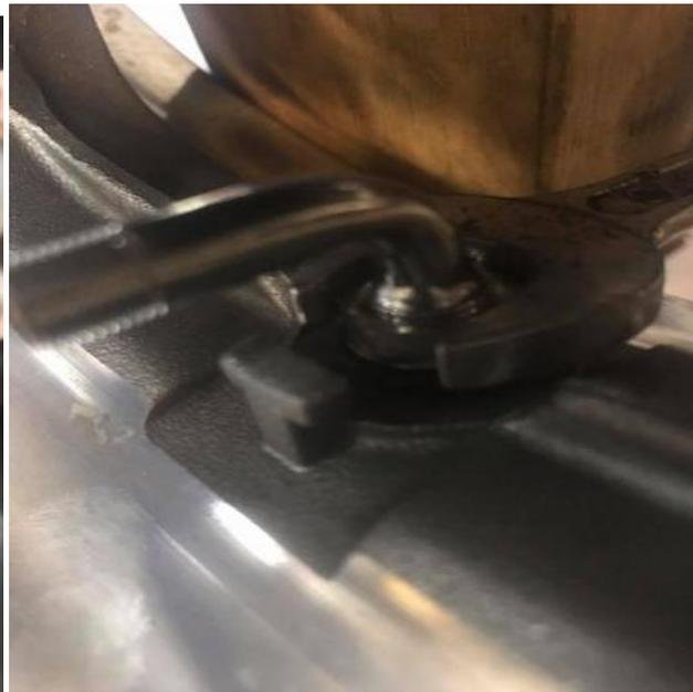
(right) Tighten the nut gently down with a 9/16" wrench don't over tighten it.
