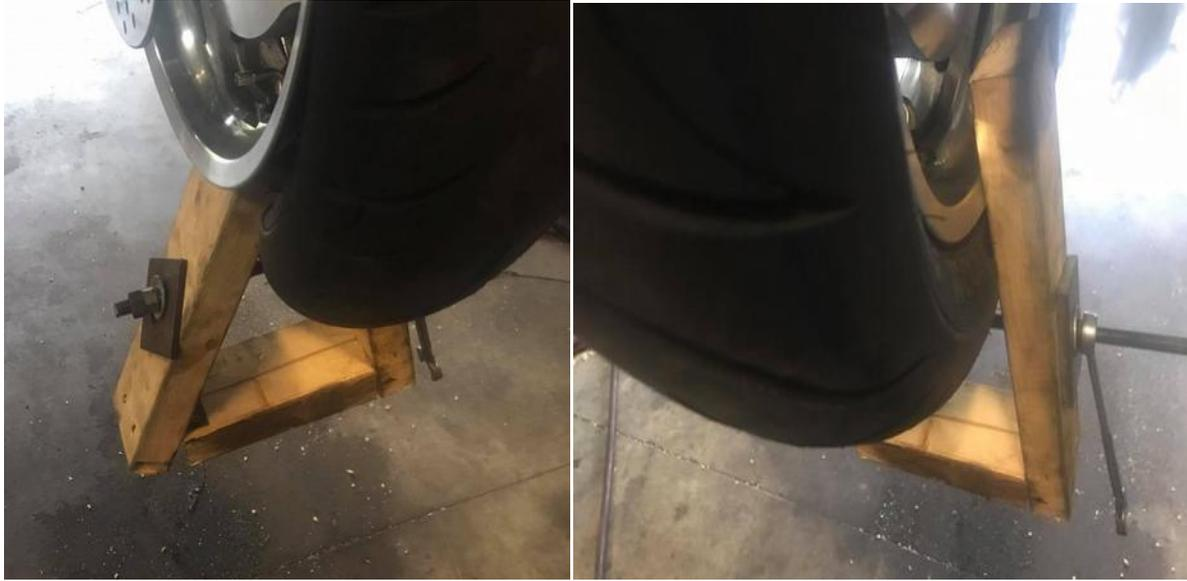
(left) I have 2 nuts together so this side I can turn with my impact wrench without the nut moving and making my socket too short
