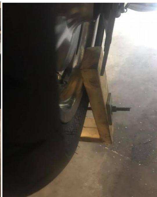
(right) The longer side goes up on the rim but below the brake rotor.
