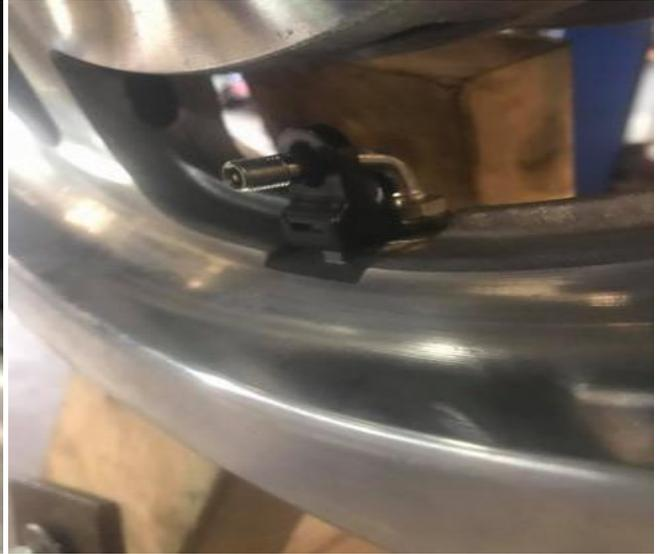
(left) Just enough to squash the rubber washer a little, there is also a rubber washer on the bottom inside the rim so it will seal without over tightening it and splitting the rubber washer.
