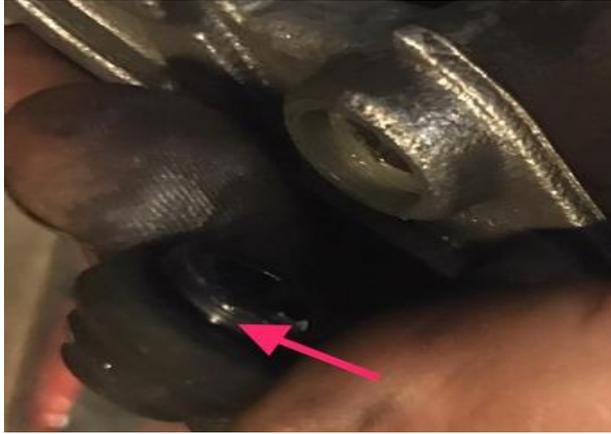
(left) Put a dab of silicone grease or dielectric grease on the end of the rubber plug so it will seal the dirt and moisture out.
