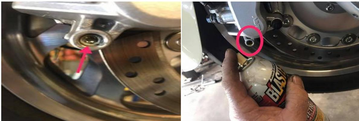
(left) After the cover screw is removed you'll find an Allen head you need to clean the head out real good so your Allen wrench will fit all the way into the head nice and tight.
