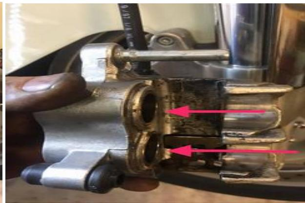
(left) If your using 2 clamps you can just tighten them down evenly as it squeezes back together but I'm using only one so have to alternate back and forth between the 2 pistons.
