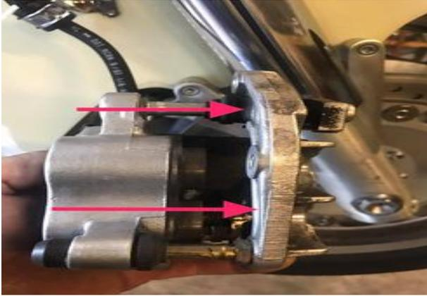
(left) Separate the 2 pieces of the caliper
