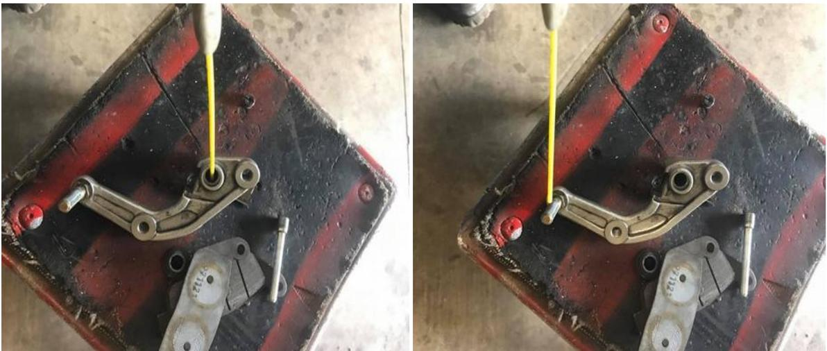
(left) After using some brake cleaner and compressed air to blow out the holes and dirt I spray some dry silicone spray in the holes and on the slide pins
