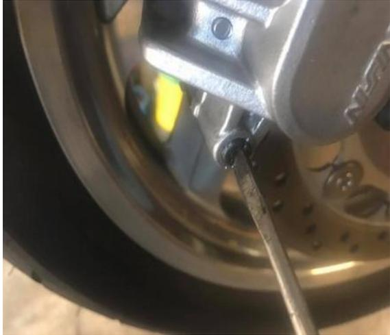
(left) Reinstall the plastic plug cap
