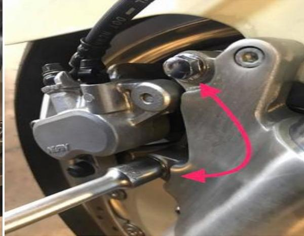
(left) Hold in tightly on the Allen wrench and give the wrench a wack to break it free. I don't remove it yet just make sure it's broke loose. Easy to have the bikes hold it while you are trying to loosen it then trying to hold it and twist it.(right) Next remove these 2- 12mm bolts and hold the caliper from falling when you remove them.
