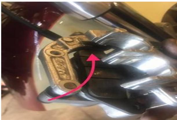
(left) Put the first pad in with the metal against the pistons, pad Part facing out and the hole where the pin came out.
