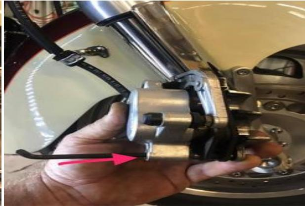
(left) Pull the caliper out from behind the mounts.
