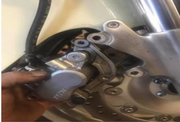
(left) Slide the caliper back into place. Be sure one pad goes on each side of the rotor so it will squeeze the rotor and you will have brakes
