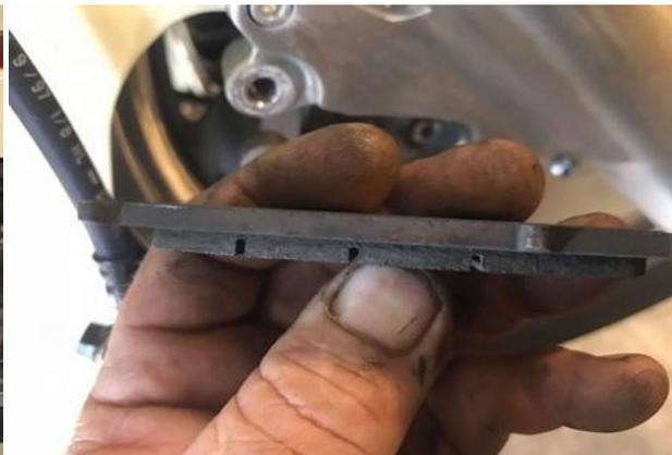
Left) hang onto the pads cause you're setting them free when you pull the pin out
