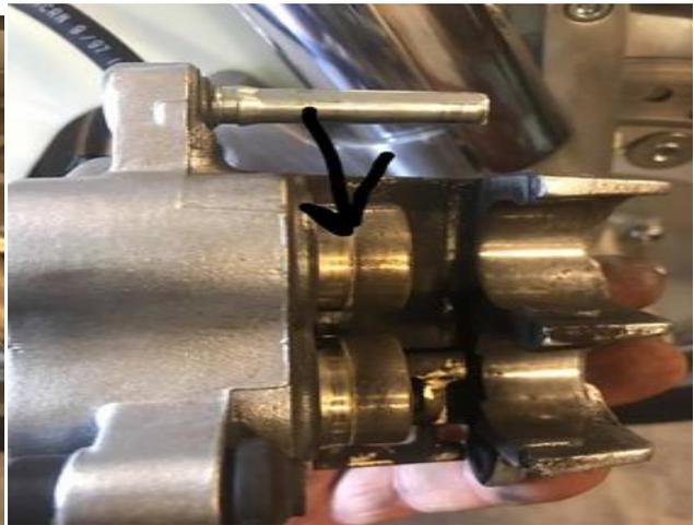
(left) Squeeze the front brake handle slowly to push the pistons out. Don't go so far you pop the pistons out but you can see the ridges where they are setting most the time about center of what you have pushed out here.
