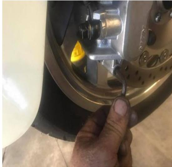
(right) Tighten the Allen head slide pin bolt up.
