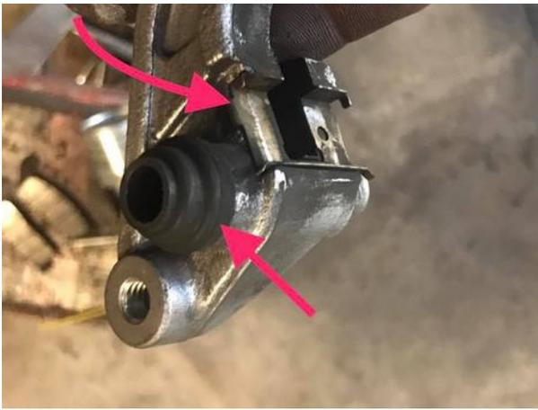
(left) Remove the rubber boot and pad clip
