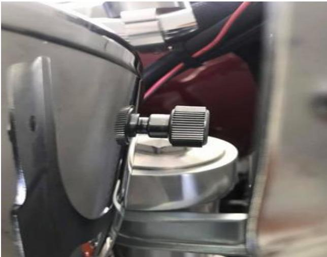
Install the trip meter knob making sure you align the flat spots.
