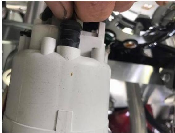
(left) Notice the flat spot here that must align with the flat spot on the knob
