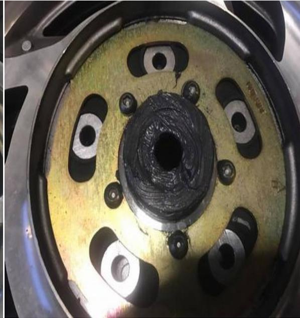
(left) Got it all clean, checked bearings and replaced O ring.
