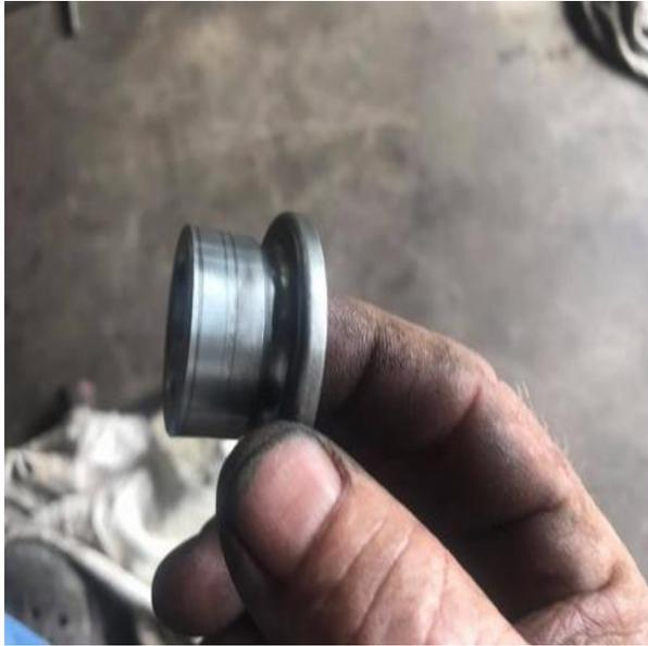
(left) Lightly grease just the end and about 1/8" of the left side of this spacer.
