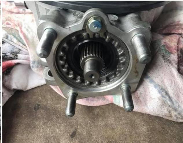
(right) Blow everything out good with air and I use a drop of blue serviceable loctite on the pinion cup stud before I slide the pinion cup on.
