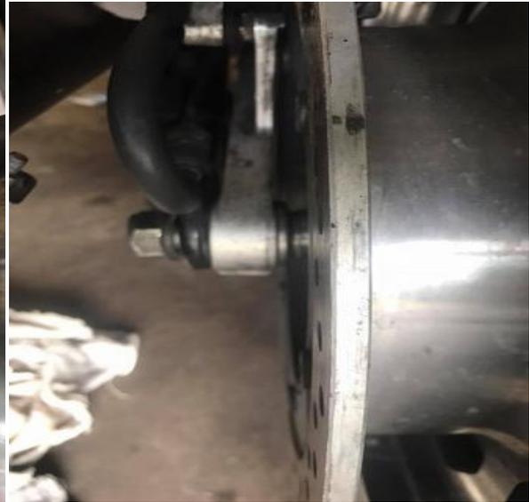
(left) Then separate the pads and slide the caliper down over the rotor
