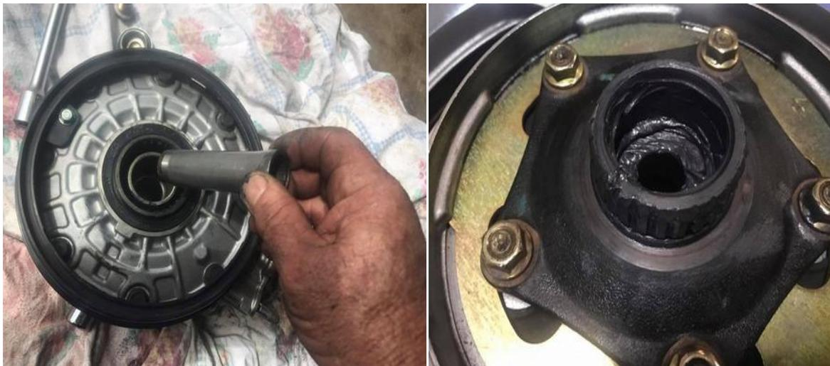
(left) Be sure you put the spacer back in and the small end to the bottom of the hole
