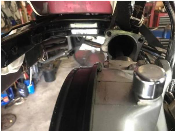
(left) Slide the final drive/ shaft up into the driveshaft tube.
