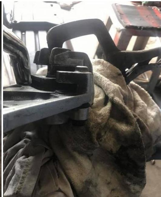
(right) I use a pair of clamp style vise grips to compress the brake pistons back. I just slide the 2 pads together and squeeze them both to compress the pistons.
