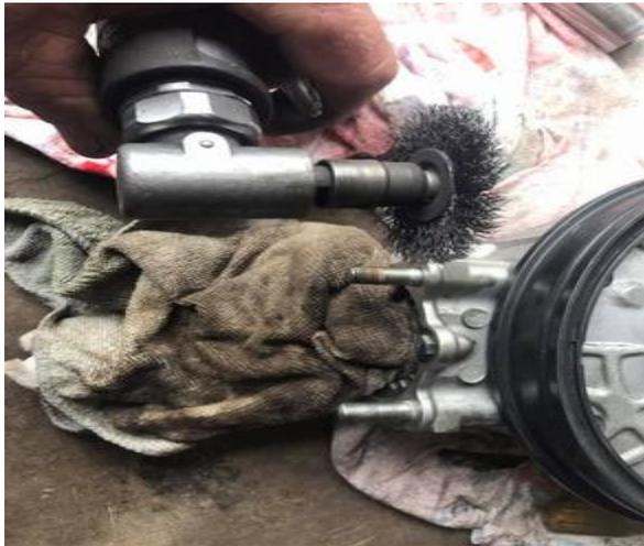
(left) Cover the area the pinion cup goes into and clean the threads on the mounting studs. If your using an air wire wheel it will take that rag away from you and wind it up.
