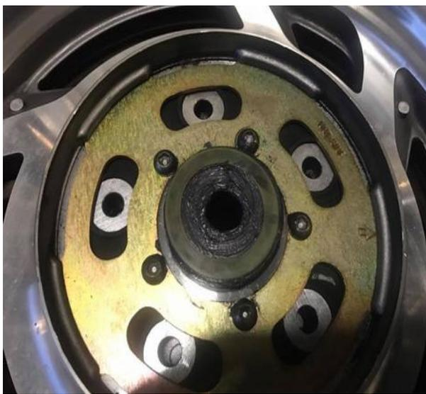
(left) Set the plastic thrust washer on the greased area
