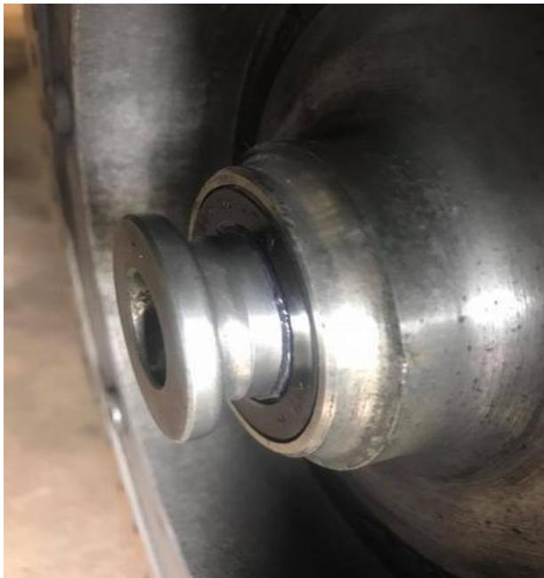
(left) Push the spacer into the seal. Now you see the reason for putting the grease just on a little bit of the end?
