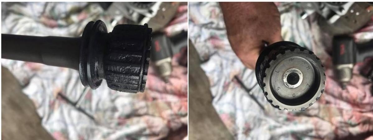
(left) Next lube the splines on the driveshaft with the 3% moly grease.
