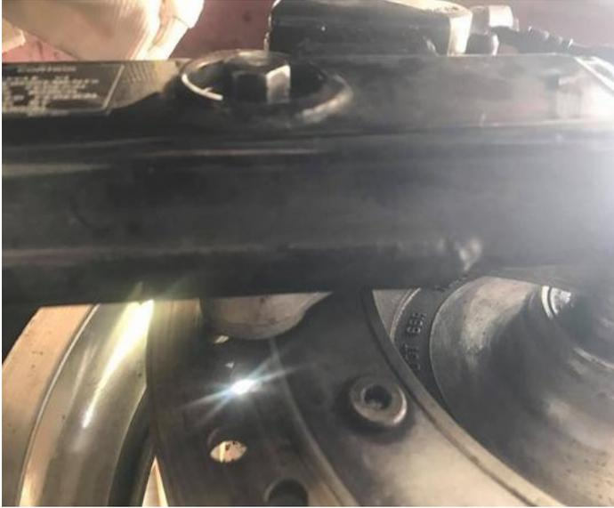
Tighten the brake slide bolt
