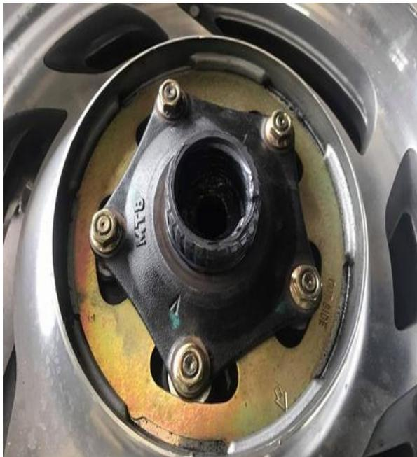
(left) Cover the splines with the lube
