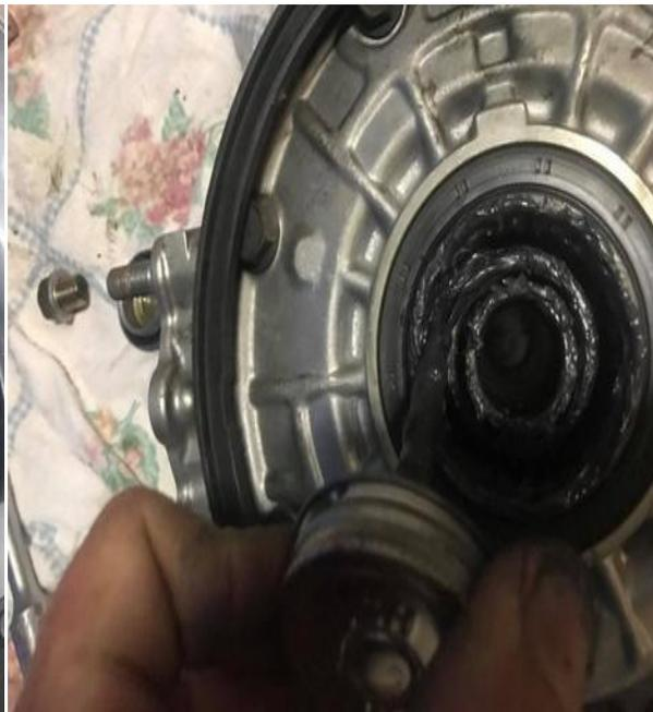
(right) Then the mating part the drive flange splines will go into. I put it in here pretty good. I was always told grease is cheaper than metal?
