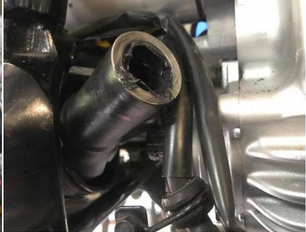
(right) Make sure you put the u joint in and hook it to the output shaft on the motor. I use some moly grease on both ends of the splines.
