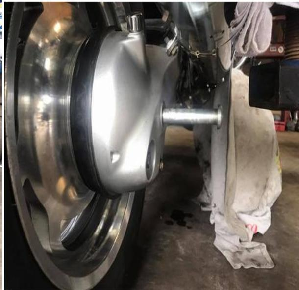
(left) I use a pry bar to help the wheel slide over evenly onto the final drive splines
