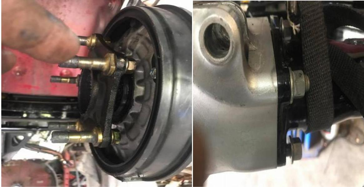
(left) put drive flange into the final drive and turn it back and forth quickly while working trying to get the final drive and driveshaft tube to come together. What is happening is the u joint is lying down against the bottom of the tube and you are jabbing the driveshaft at it trying to get the hole and splines to all line up.
