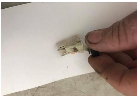
(left) Hold the bottom and lift the button out. Do this on an area that if the little ball comes out you can find it. Doesn't always pop out but when it does, the hunt is on.
