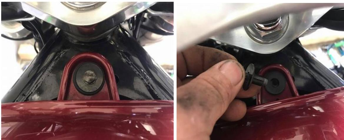
(left) Then remove the 8mm bolt at the front of the tank
