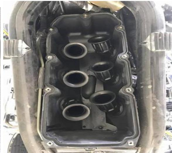
(right) Make sure the gasket around the edge is in place when putting it back together.
