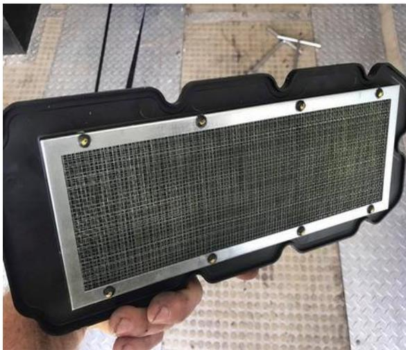
(left) This is the bottom side of the filter that goes down toward the engine when you replace it
