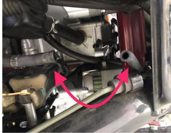
(left) This is a Pingel petcock that will be used on this bike along with a Dan-Marc electronic fuel shut off. The Petcock is non vacuum and only requires one line, the fuel supply line.
