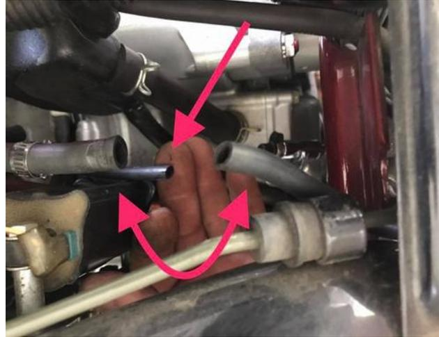
(left) This is the OEM style petcock, the large fitting on the left goes to the fuel supply line and the smaller fitting on the right goes to the vacuum line come off the #6 cylinder intake runner.
