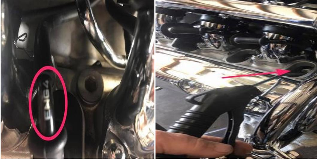
(left) Each plug wire is marked as to what cylinder it goes to. On the left side of the bike you have starting from the front of the bike going toward the rear 2,4,and 6 cylinders. On the right side you have 1,3 and 5.
