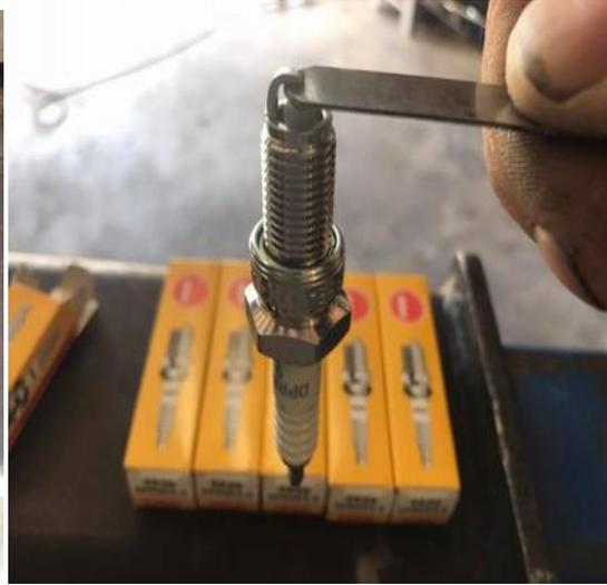
(right) A wire gapping tool works a little better but mines hiding with all the 10mm sockets I reckon? So don't force it in but don't make it loose and wobbly just snug fit.
