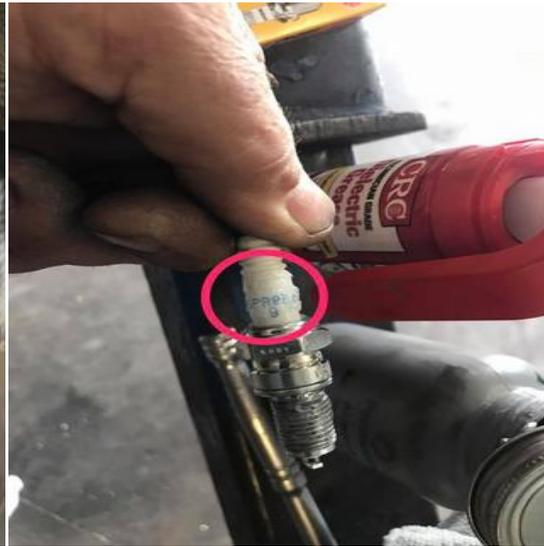
(right) I put a little dielectric grease around the ceramic part just before the metal so when the boot gets pushed on it will seal the boot around the plug and also let it slide back off easily when it comes time to remove it again.
