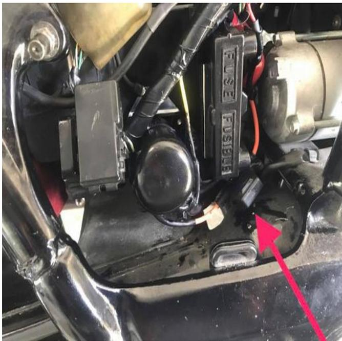
I applied a liberal amount of dielectric grease to all the connections then slid the rubber cover over the solenoid and ran a zip tie around it to hold it from falling off. Now the 30 amp main fuse is in easy reach inside the covered fuse holder filled with dielectric grease.
