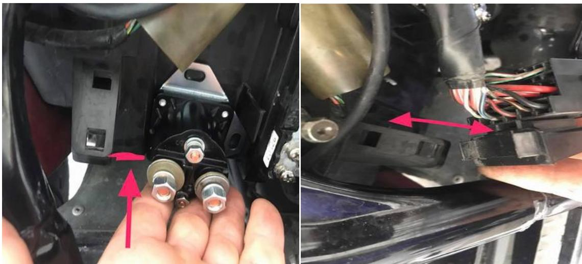
(left) I held it flush with the bottom of the battery box with the terminal with the "S" at the top
