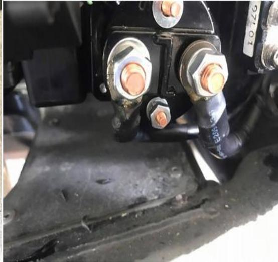
(left) Installed bigger ring terminals, soldered and heat shrink.
