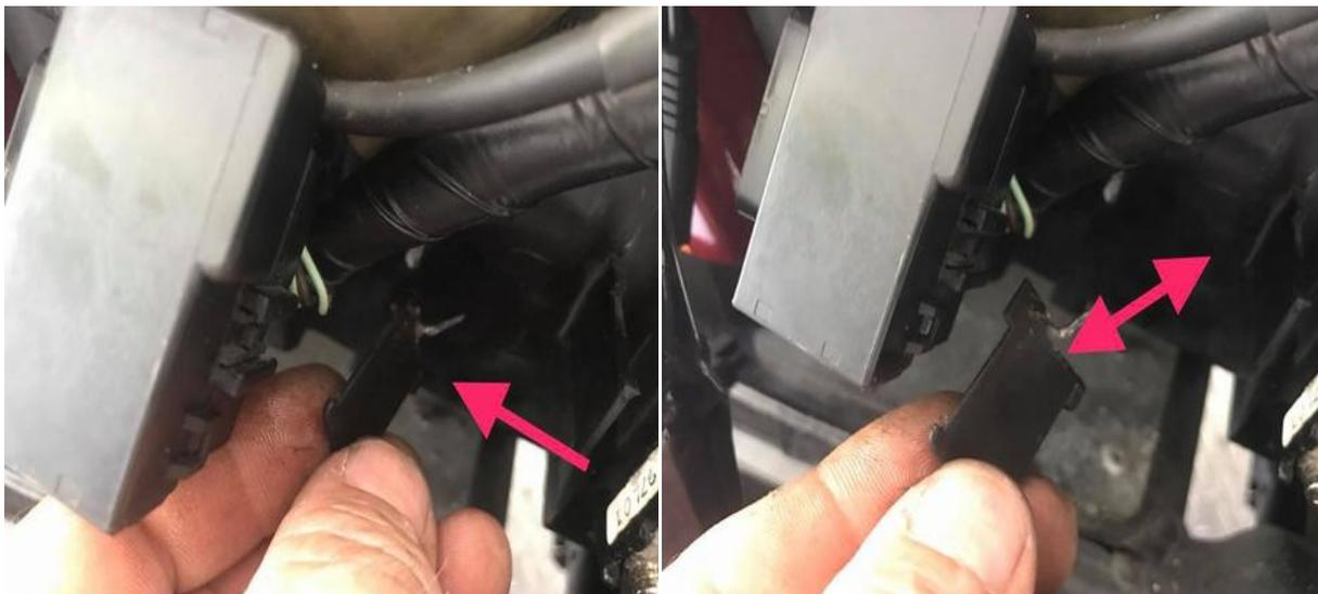
(left) Got to remove a couple plastic pieces that were used to hold the old solenoid
