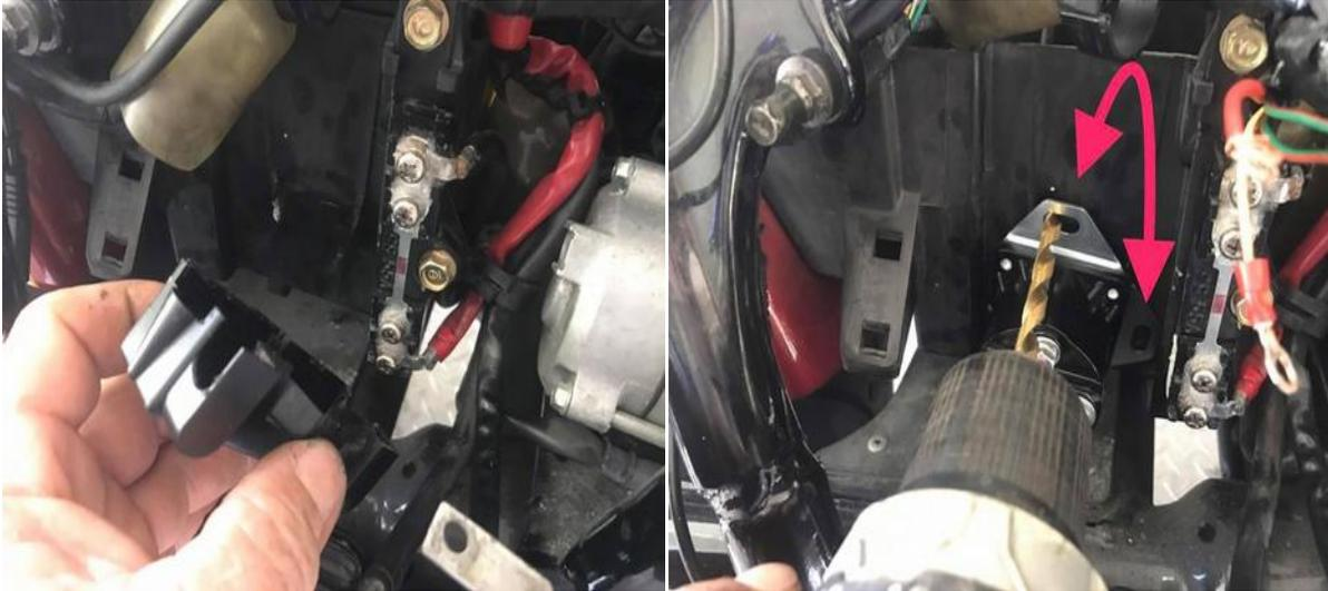
(left) Pulled the cap off the 50amp fuse holder
