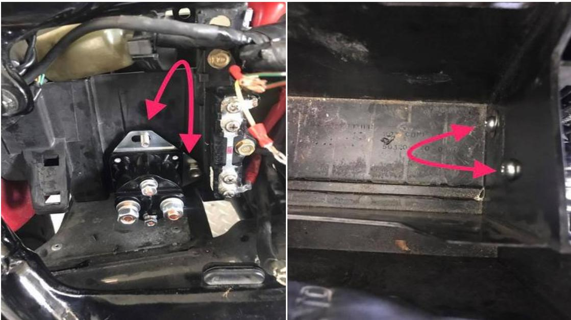
(left) I used 2 - 3/4"X 1/4" Phillip head bolts pushed out from the inside of the battery box and nuts on the outside to hold the solenoid.
