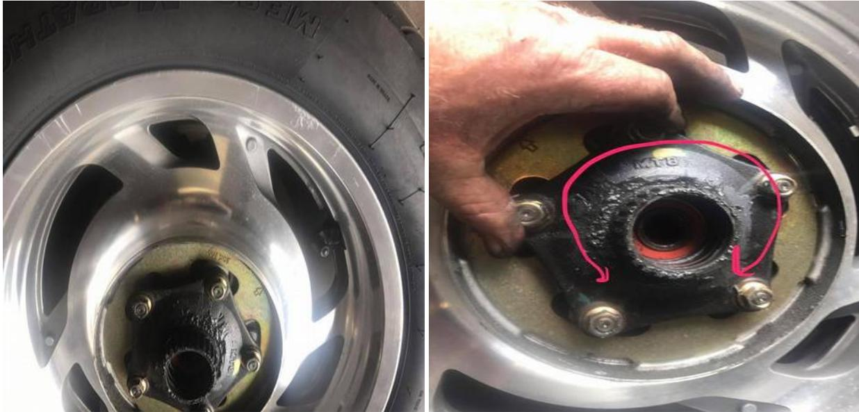
(left) Got the wheel off and notice quite a bit of grease leaking out around the splines. My first thought was the last guy didn't change the 3 o rings?(right) Trying to work it back and forth to see if there is any wear or movement in the wheel dampers. These are really tight.
