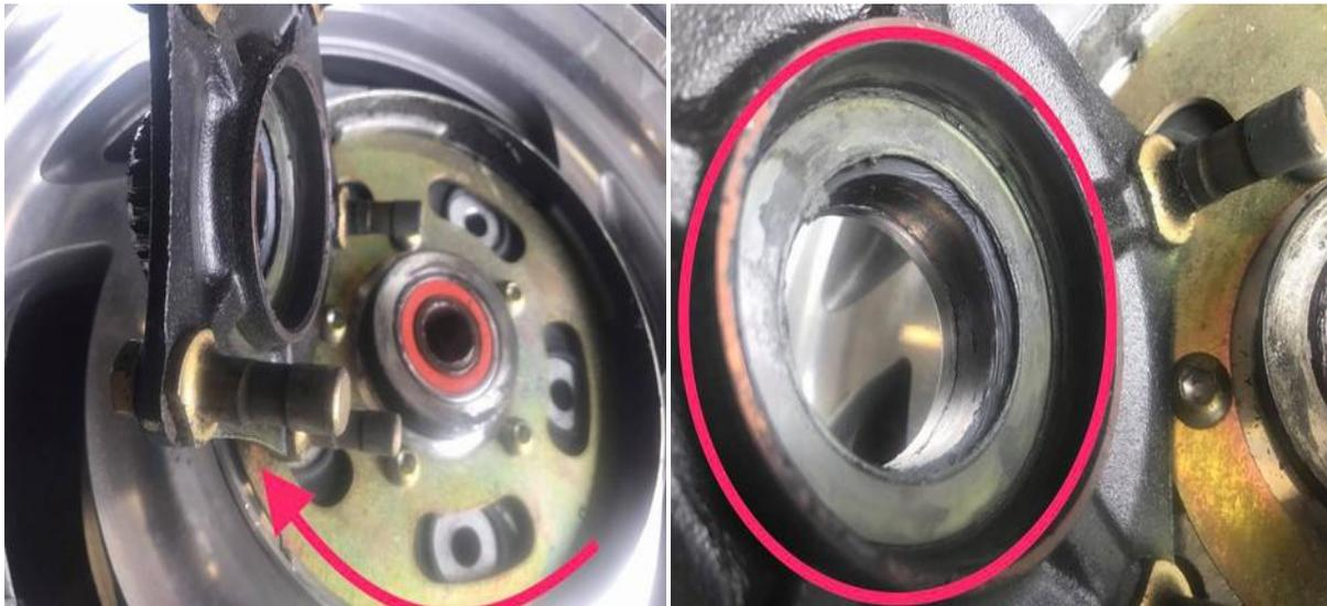
(Left) Pins were really dry which made it hard to get the drive flange off. The pins seat into the wheel dampers to cushion the jerk on and off the throttle. The dampers are about \$35 for new ones and very easy to change but these are really good.(right) The thrush washer is here and need to be sure it goes back on, if it shows wear replace it. I do mine every other tire change.
