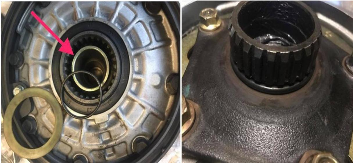
(left) Put a little grease on the new o ring and put it on the shaft in the groove at the top
