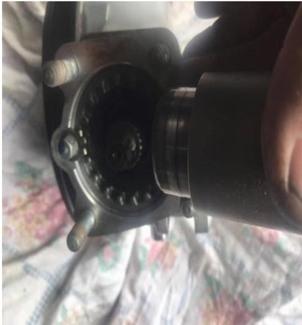
(left) Once the nut is removed you can pull the pinion cup off
