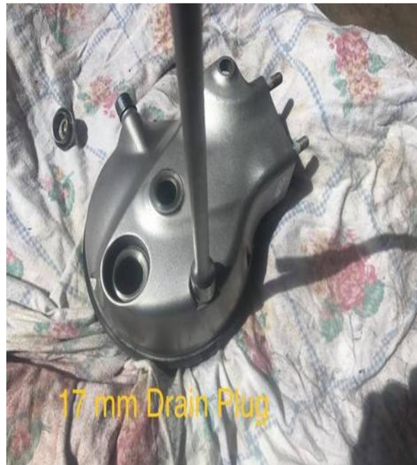
(left) Remove the fill plug with a 17mm socket
