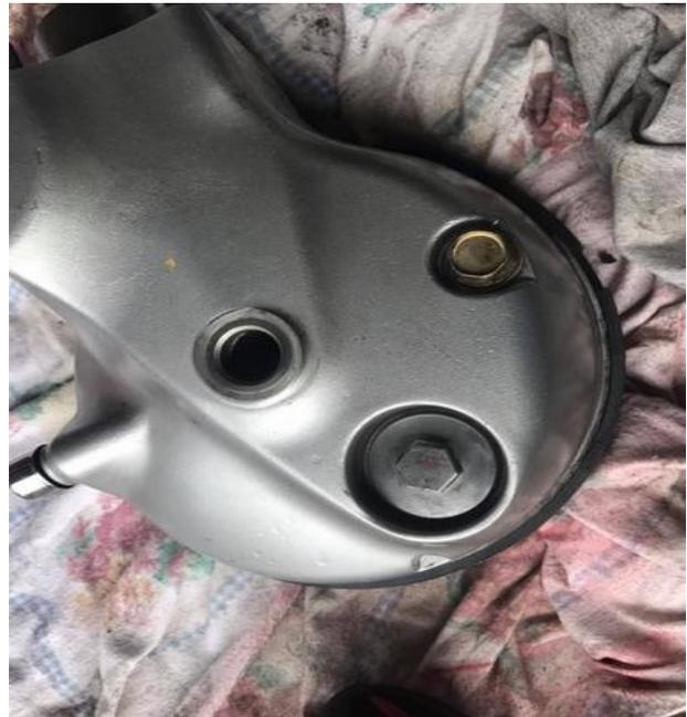
(left) I put a dab of oil on the o ring before I install it back on
