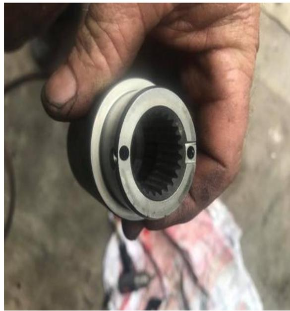
(left) Clean the cup up real good and be sure the holes are open and clean.
