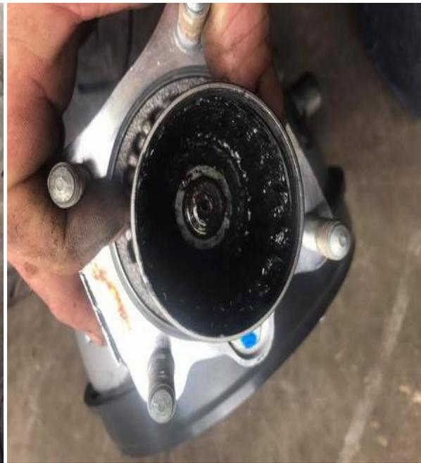
(left) After pulling the driveshaft out of the final drive I inspect the shaft and pinion cup splines.
