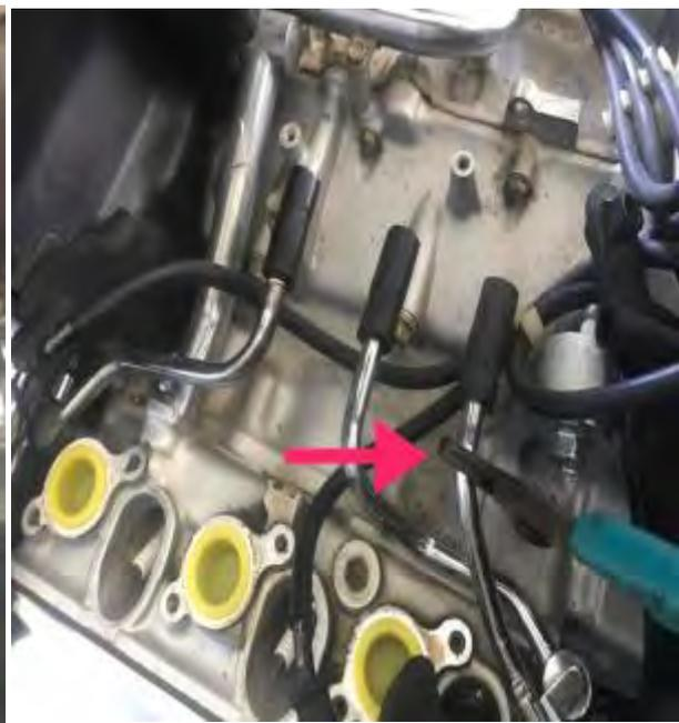
(left) On the kits you buy they have a block off plate that replaces this fitting on the end of the chrome tube. We are keeping the chrome so not doing that.
