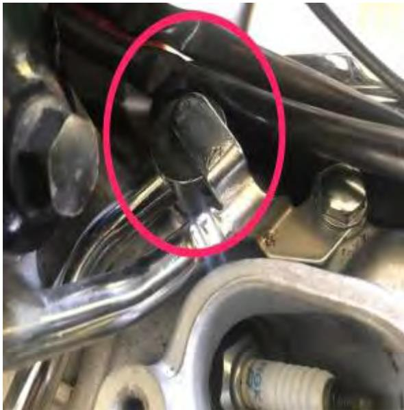
(left) Tab bent down and bolt reinstalled
