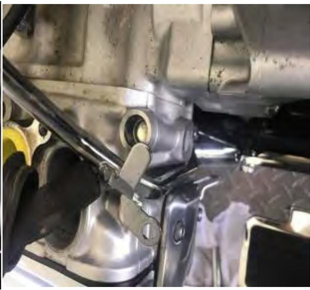
(left) Back left side pull the tube out and drive the next freeze plug in.
