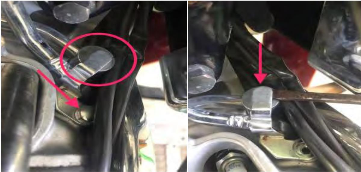
(left) The front right tube is a little harder to get out. Remove the bolt.
