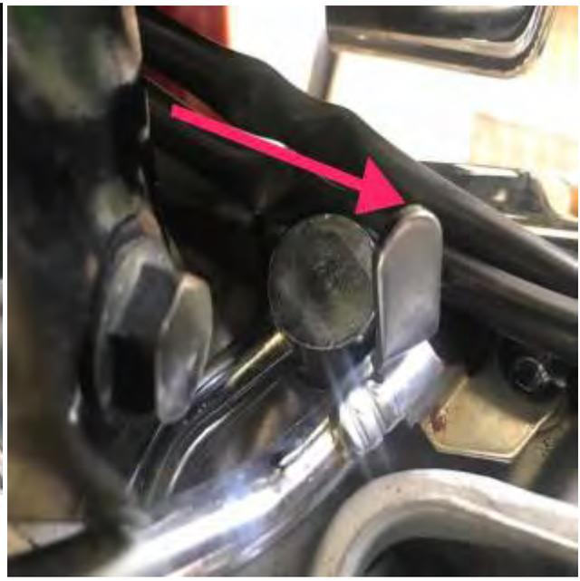
(right) Fold the tab back down over the cap after grinding the cap to fit in tight.
