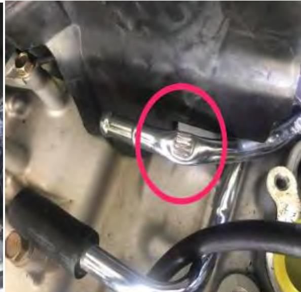
(Left) The front right side tube that comes up from the bottom we are going to crush the tube behind where the intake runner will hide it
