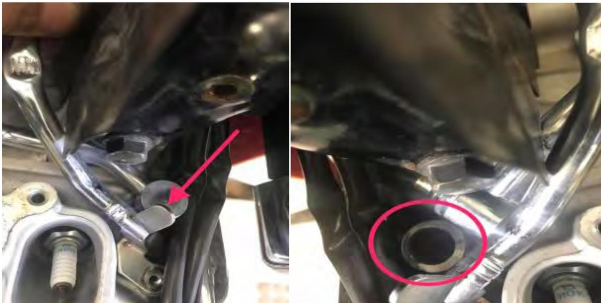
(left) Bend it all the way out of the way so the tube can be removed
