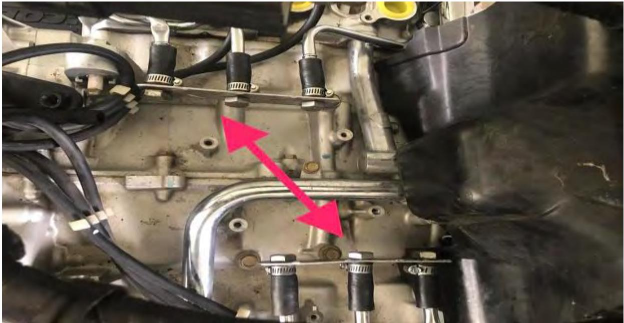
Finished product used the existing rubber tubes that were hooked to the pair valves and stick a bolt thru the plate and into each hose and put a clamp on it. Could probably almost just use the bolts and plates to do the de-smog? One of the guys on here has done it that way and it looks really good. Anyway, a lot less clutter on the engine, less problems down the road, no worries of popping on de-cell. Choice is y'all's if you do it or not?
