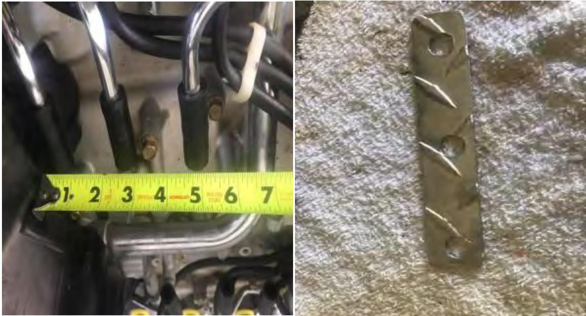
(Left) Measuring for a plate and holes. Gonna make a plate 5 1/2"X 1" wide and drill 3 holes to match each tube.
