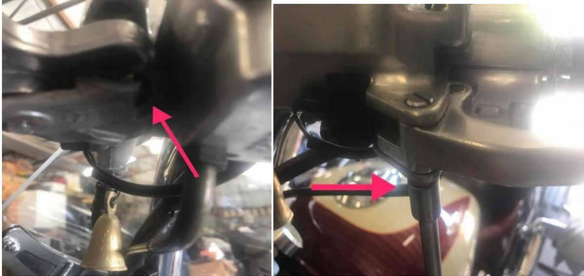
(left) Check to make sure the rubber boot isn't binding.
