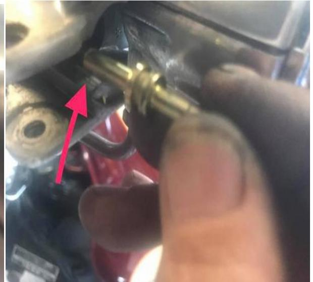
(left) Need to remove the plunger rod that goes into the master cylinder.
