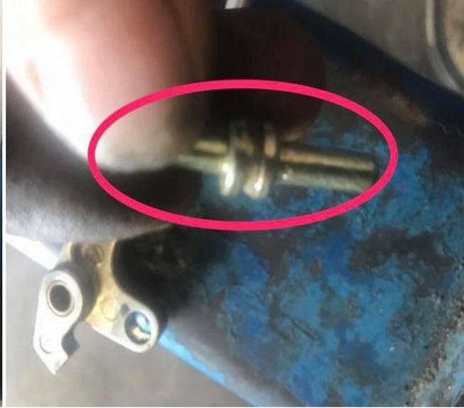
(left) I'm using a silicone grease to lube the pivot parts and bushings.
