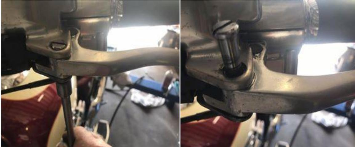
(left) Remove the 10mm nut off the pivot bolt
