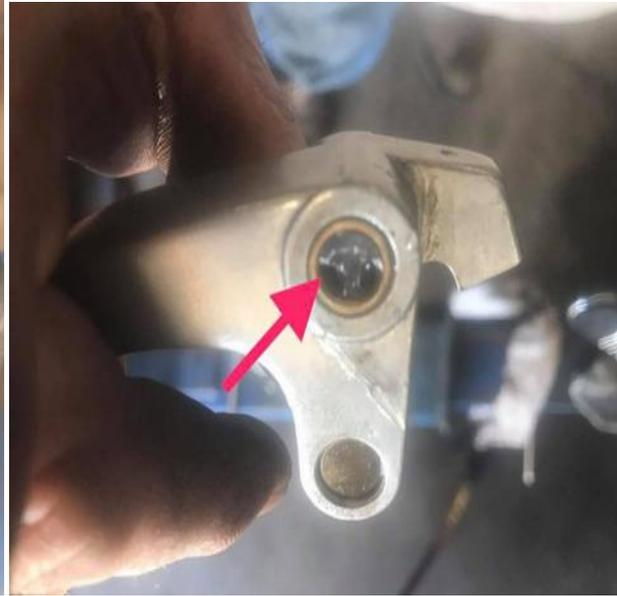
(right) Lube the top side of the handle holes so when the pivot bolt is installed it will push the lube on down through the rest of the bushing.
