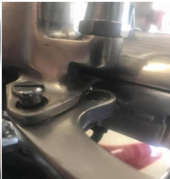
(left) Insert the pivot bolt in the hole. If the threads don't want to line up squeeze the Clutch handle a couple times to push the plunger into the master cylinder so it will seat.
