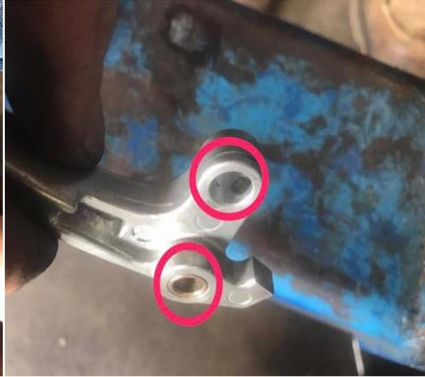
(left) Slide it all the way thru so it looks like this. Spin the handle around on the sandpaper so it will clean the corrosion and dirt off the inside of the hole.
