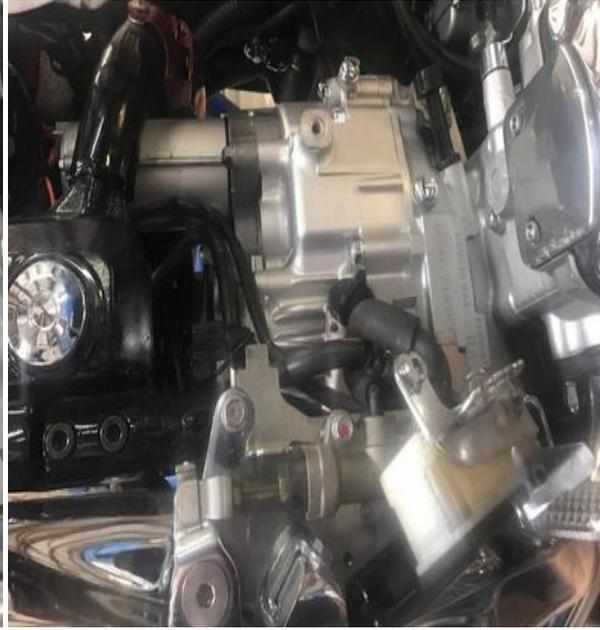
(left) Remove the rear brake master cylinder cover and mounting bolt. (right) Swing it down out of the way.
