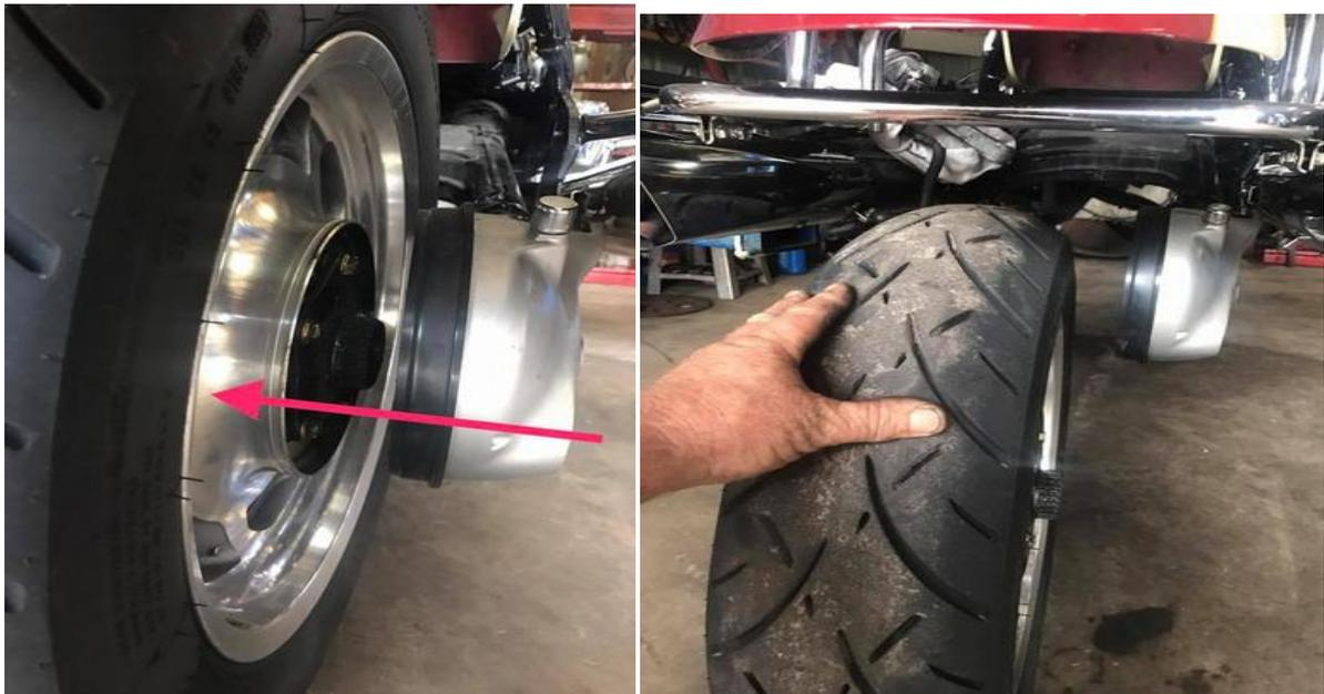
(left) Pull the wheel to the left side until it comes out of the final drive splines
