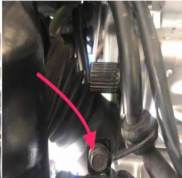
(left) Push the boot forward and then push the u joint back off the output shaft.
