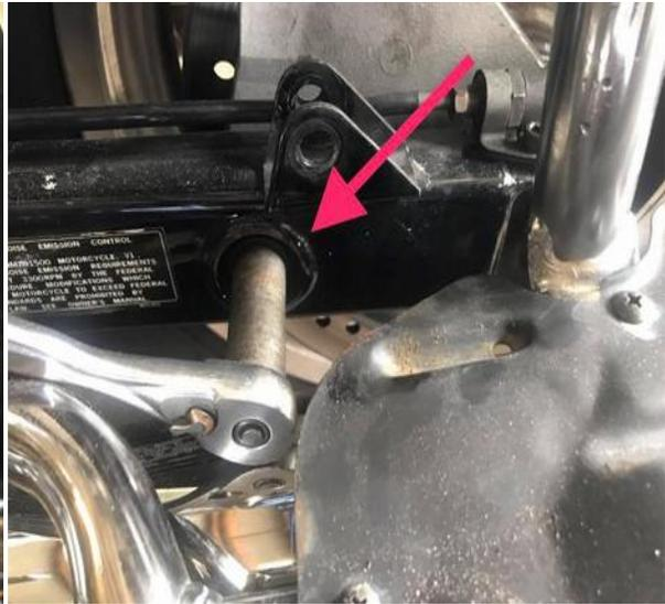
(left) Then I loosen the top driveshaft housing nuts. I don't remove them just loosen them so they still have a few threads left before coming off
