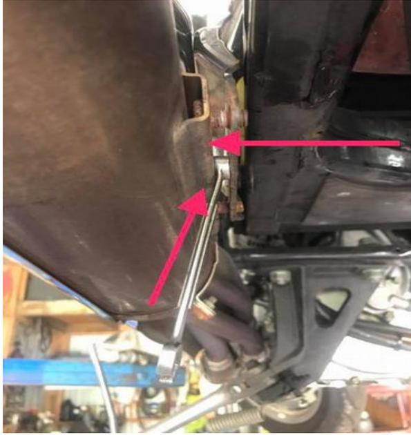
(left) I pry the mufflers out and stick a box end wrench in between the hanger and muffer to shim it out away from the swing arm slightly.
