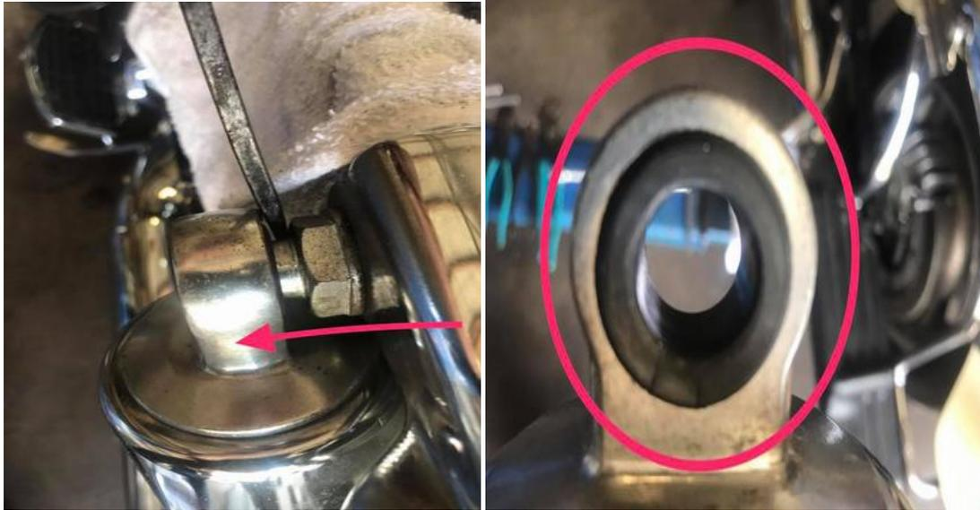
(left) Pry the top of the shock off the frame stud. It helps to take some of the weight off the wheel so it isn't under pressure and will come off easier.
