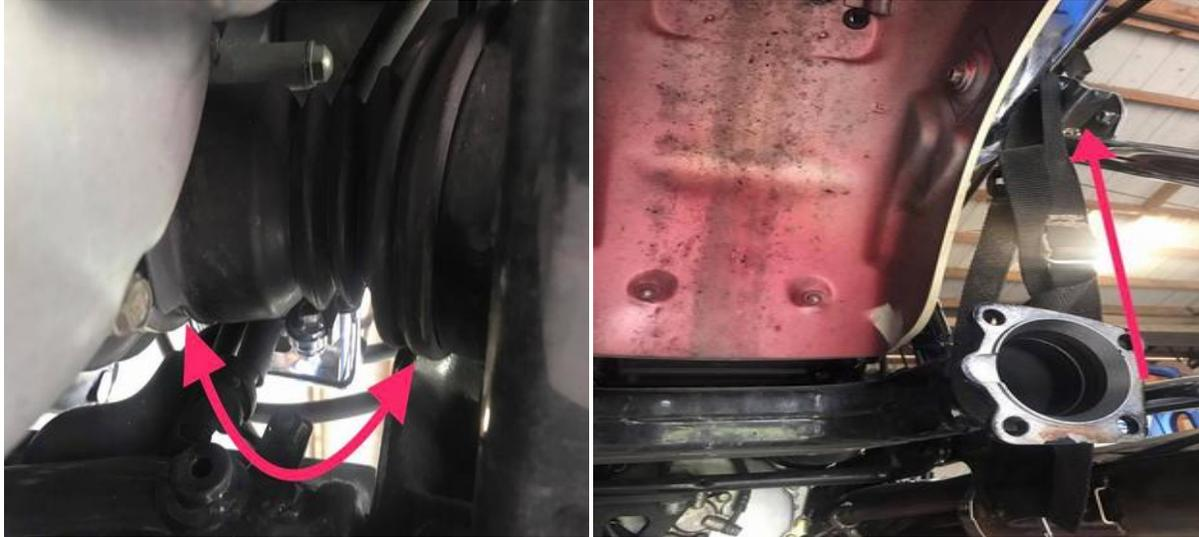
(left) Next push loosen both ends of the u joint boot, push it back away from each end so it's just floating
