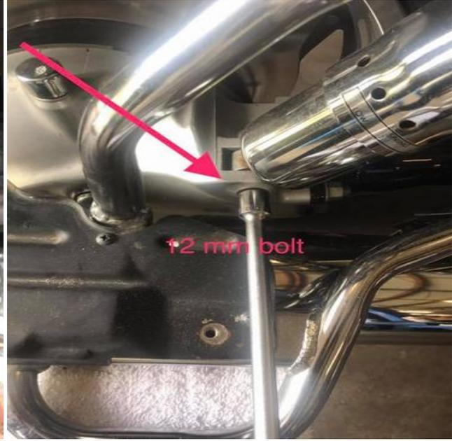
(right) With the weight of the bike on the rear wheel and bags removed I remove the bolts from the shock bottoms.
